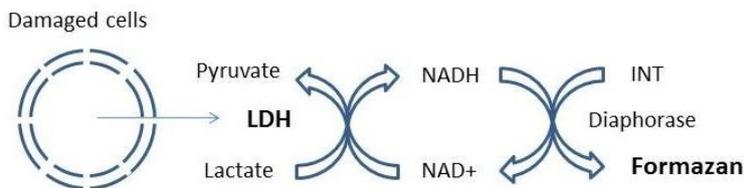
Figure :Schematic diagram of LDH Cytotoxicity Assay Kit
